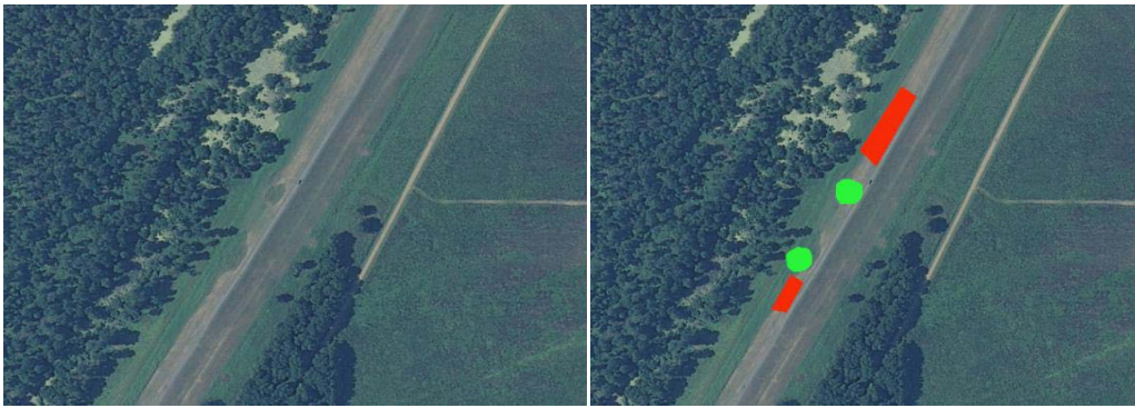
Figure 3.8 Subset of levee. Left Image: Actual levee segment. Right Image: Mask segment. Green: landslide; Red: healthy levee.
