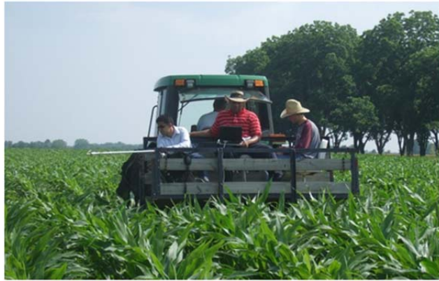
Figure 4.7 Image of collection of handheld hyperspectral data mounted on a tractor.
